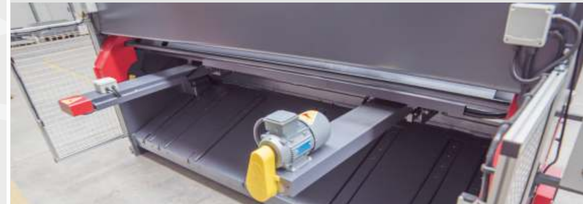
Motorized Back Gauge has \pm 0,1\text{mm} Accuracy
